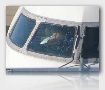
At three plies thick, glass windshields are designed to protect against bird strikes; de-ice from minus 50 degrees; resist fogging and provide exceptional optical qualities.
