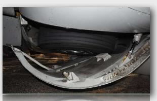
accident, concluding that debris in the gear-door actuator caused the jam.
